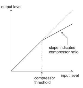
The *compressor threshold* is the level point in dB above which the audio gain will be reduced. On the Stereo Toolbox this can be varied from 0 to 20 using the **DRIVE** control (9). Turning the control clockwise (from 0 towards 20) lowers the threshold and increases the amount of compression.
